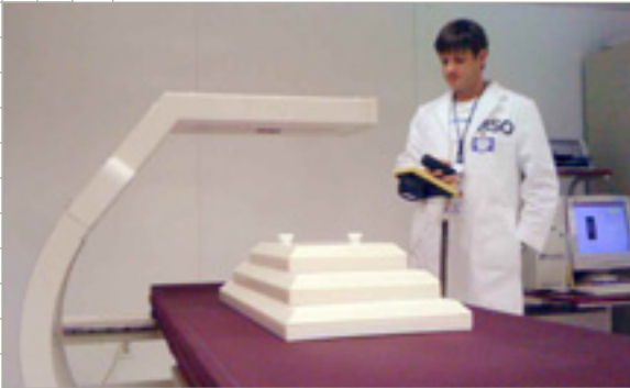
Radiation specialist Daryn Bovard conducts an inspection on a dual-energy X-ray absorptiometry unit using an ion chamber.
