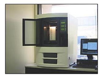
The Studio boasts a Stratasys Dimension printer that produces functional ABS plastic 3-D models from CAD files.
