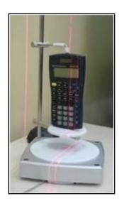
The NextEngine™ Desktop 3-D Scanner generates high definition 360° surface scans of objects. Using Studio software, surface scans can be used to build digital solid objects that can be "printed" in the 3-D Printer.
